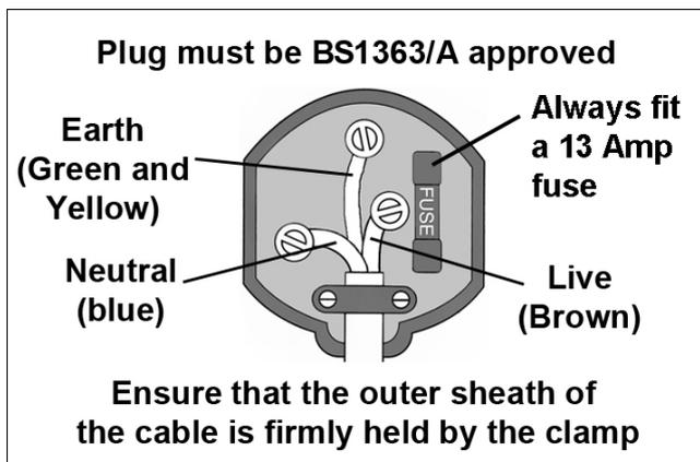
The fuse in the plug must be replaced with one of the same rating and this replacement must be ASTA approved to BS1362.
